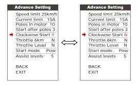
**8.17 Throttle 6KM**: this parameter can set the throttle function, N represent max speed, Y represent 6Km.
