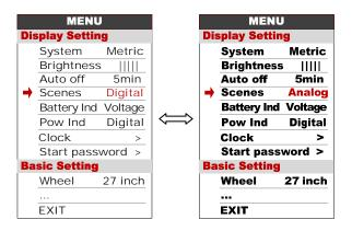
**8.5 Battery Ind**: Press UP/DOWN button to change the battery indicator, Voltage / Percentage / OFF.
